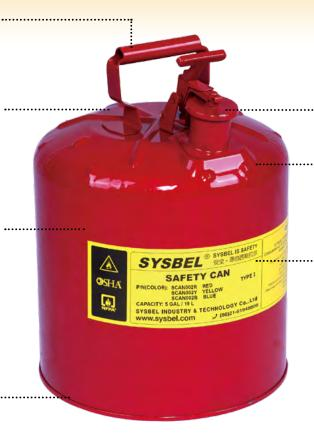
Positive press relief cap, leaktight, automatically vent vapor between 0.2 and 0.35bar(3 and 5 psig) to prevent rupture(or explosion in event of fire), spring loaded, it closes automatically after filling or pouring
